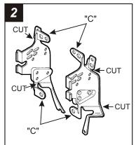
Locate Radio Housing "C". dotted lines as a guide, cut and remove all tabs on the Mounting Brackets EXCEPT tabs "C". Skip to the Installation Instructions for ALL VEHICLES on Page #2.
