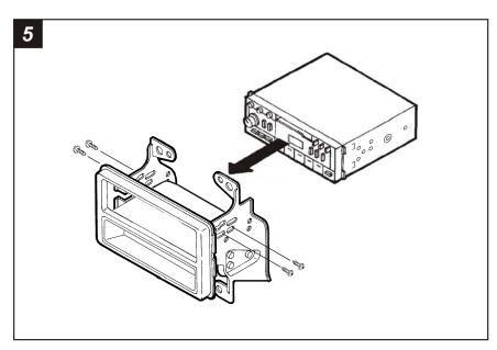
Align the holes in the Mounting Brackets with the holes in the ISO-DIN head unit and mount the Brackets to the head unit with the screws included with the unit.
