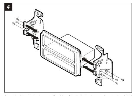
Attach the Mounting Brackets to the sides of the Radio Housing by inserting the slotted Bracket tabs into the slotted Housing tabs. (Be sure the mounting bosses on the Brackets align with the mounting bosses on the Pocket ). Mount the Brackets to the Pocket with (6) #6 x 1/4" Phillips Flat-Head Screws.
