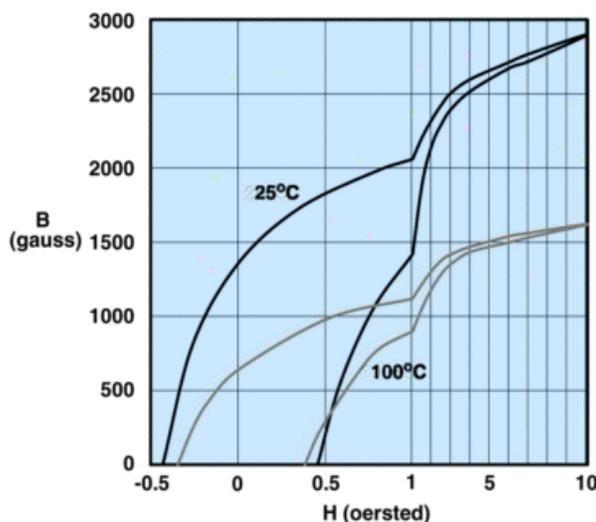
Measured on a 17/10/6mm toroid at 10kHz.
