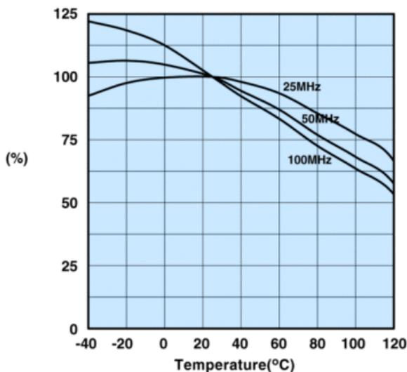
Measured on a 2643000301 using the HP4291A.
