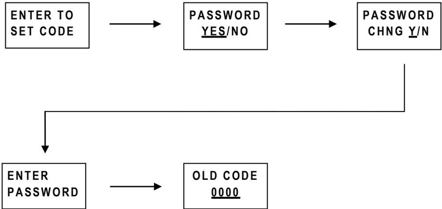
2. Using the function keys, press UP or DOWN to select "YES" or "NO". Press enter to confirm the selection. A confirmation screen will appear select "Y" to set the password or "N" to go back.
