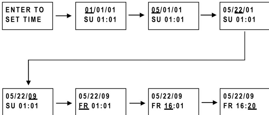
2. Using the function keys, press UP or DOWN to enter in the correct month, date and year.
