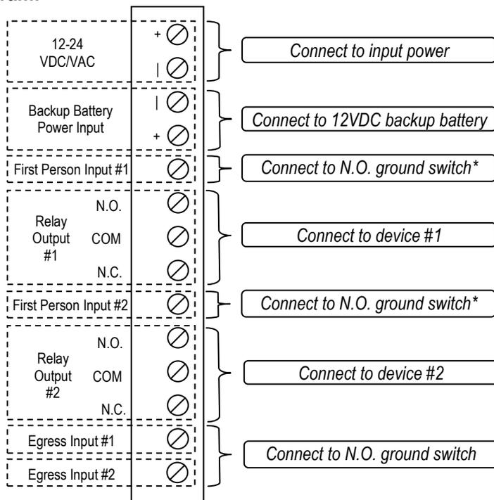
\* The First Person Input function suspends the operation of the SA-027Q annual timer. If a relay is turned on before the first man feature is activated, the relay will remain on until the first man feature is deactivated. Once deactivated, the timer will turn on the last programmed function prior to the first man activation.
